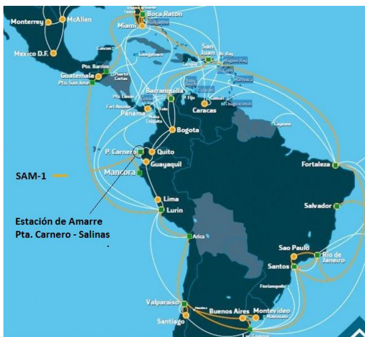
Figura 3. Cable Submarino SAM-1
